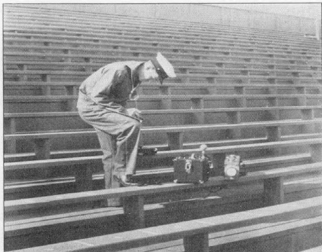
FIGURE 6. Showing the sound-level meter and oscillograph as used in measuring the over-all characteristic of the system.
